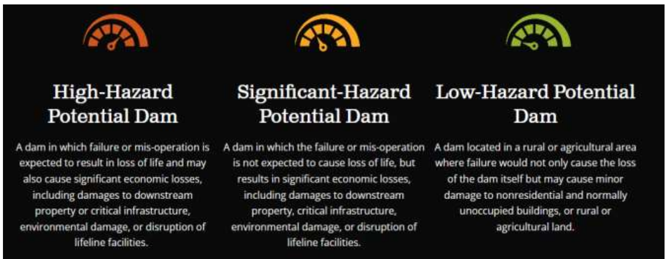
Figure 9-1. Dam Hazard Potential Classifications
